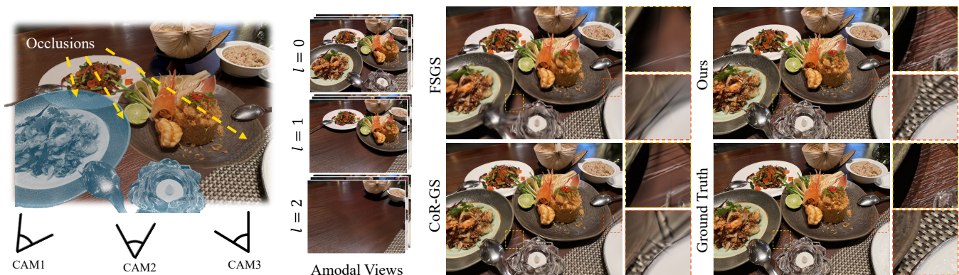
Figure 1: Visualization of STO-GS. Given sparse modal views (left), we generate layered amodal views (middle) to reveal occluded content and guide opacity-aware training for reconstructing hidden regions. As shown in the rendered comparisons (right), STO-GS outperforms prior methods (FSGS [43], CoR-GS [41]) in both geometric and visual consistency, especially for occluded, non-central areas.
