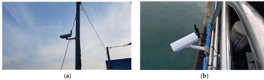
Fig. 4. The speed camera modules installed (a) on the berthing area and (b) where the ship is entering.
