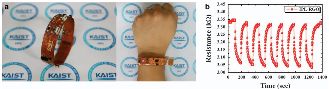
Figure 9 (a) Optical image of the wearable sensor module integrated with the intense pulsed light-reduced graphene oxide (IPL-RGO) sensor (blue dotted box). (b) Dynamic resistance transition of the IPL-RGO sensor on the wearable sensor module to 20 p.p.m. of H 2 S at room temperature.
