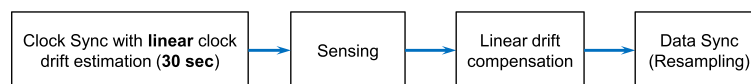
Figure 5. A two-stage time synchronization strategy based on linear clock drift compensation (stage 1) and resampling (stage 2).
