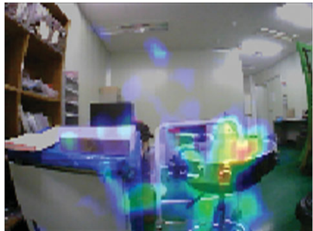
Figure 13. Compton image of 10-kg DU source 90 cm in front of detector. Imaging time: 10 min.
