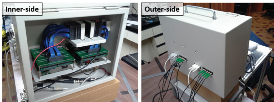
Figure 7. Compton imaging system developed in the present study.
