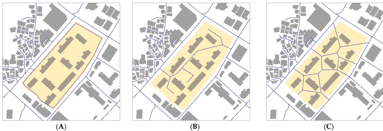
Figure 3. Three different scenarios of internal pedestrian network of apartment sites and their connection to surrounding neighborhoods: (A) Gated; (B) Partially opened; (C) Fully opened with Voronoi modification.
