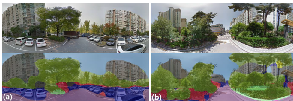
Fig. 4. GSV segmentation result of trained FCN8s GVI: 31.29 (a), 43.01 (b).
