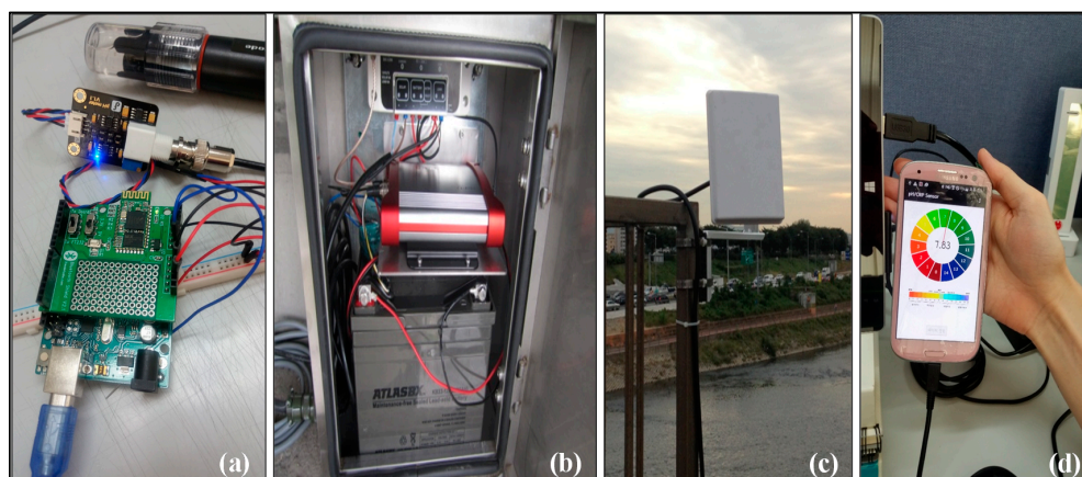
Figure 3. (a) Integrated Arduino-based Bluetooth shield pH sensor; (b) solar power-controlled battery (3 V to 5 V with 12 V to 24 V); (c) Bluetooth flat panel antenna (2.4 GHz with 15.5 dBi); and (d) Arduino-based mobile application for smartphones.
