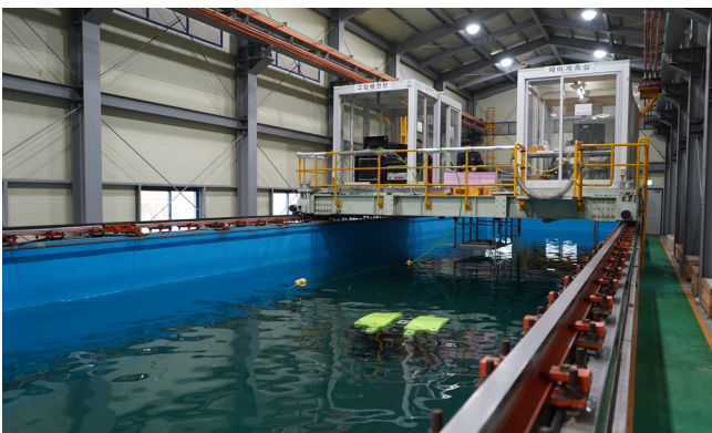
Fig. 9 Scene of water tank test with KRISO ROV
