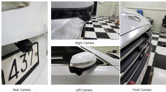
FIGURE 22. AVM camera installation.
