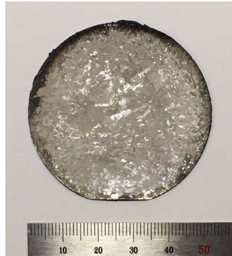
Fig. 1. Image of a 2-inch bulk GaN grown by HVPE.
