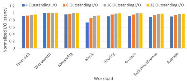
FIGURE 7. Normalized I/O latency of eight-channel, eight-way configuration.
