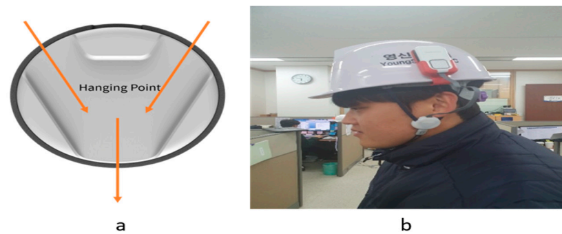
Figure 7. Type C PPG sensor: (a) the sliding design of the sensor; (b) prototype of the Type C sensor.
