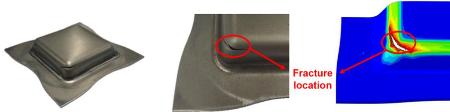
Fig. 12. Fracture region from the test and the finite element analysis.
