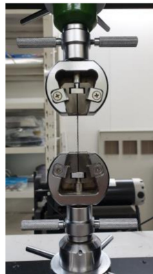
Figure 5. Monotonic tensile test setup.
