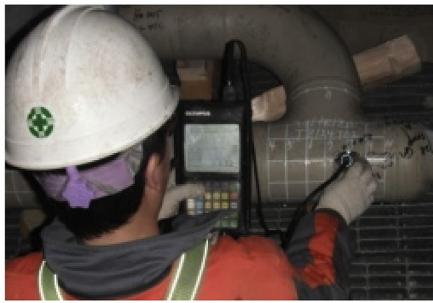
(b) UT inspection during a plant outage
