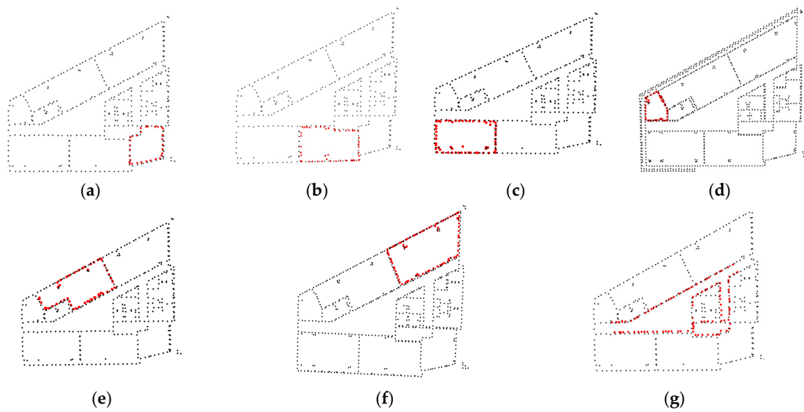
Figure 19. Coarse registration results: (a) 301A, (b) Room 301, (c) Room 302, (d) Room 303, (e) Room 304, (f) Room 305, and (g) Hallway.
