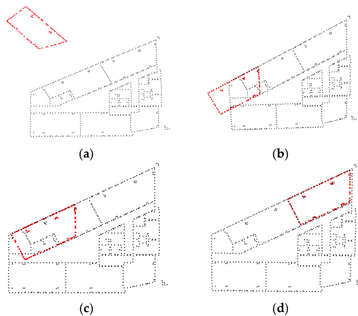
Figure 9. Rotational and translational alignment: (a) initial state of models, and (b–d) search sequences of coarse registration.
