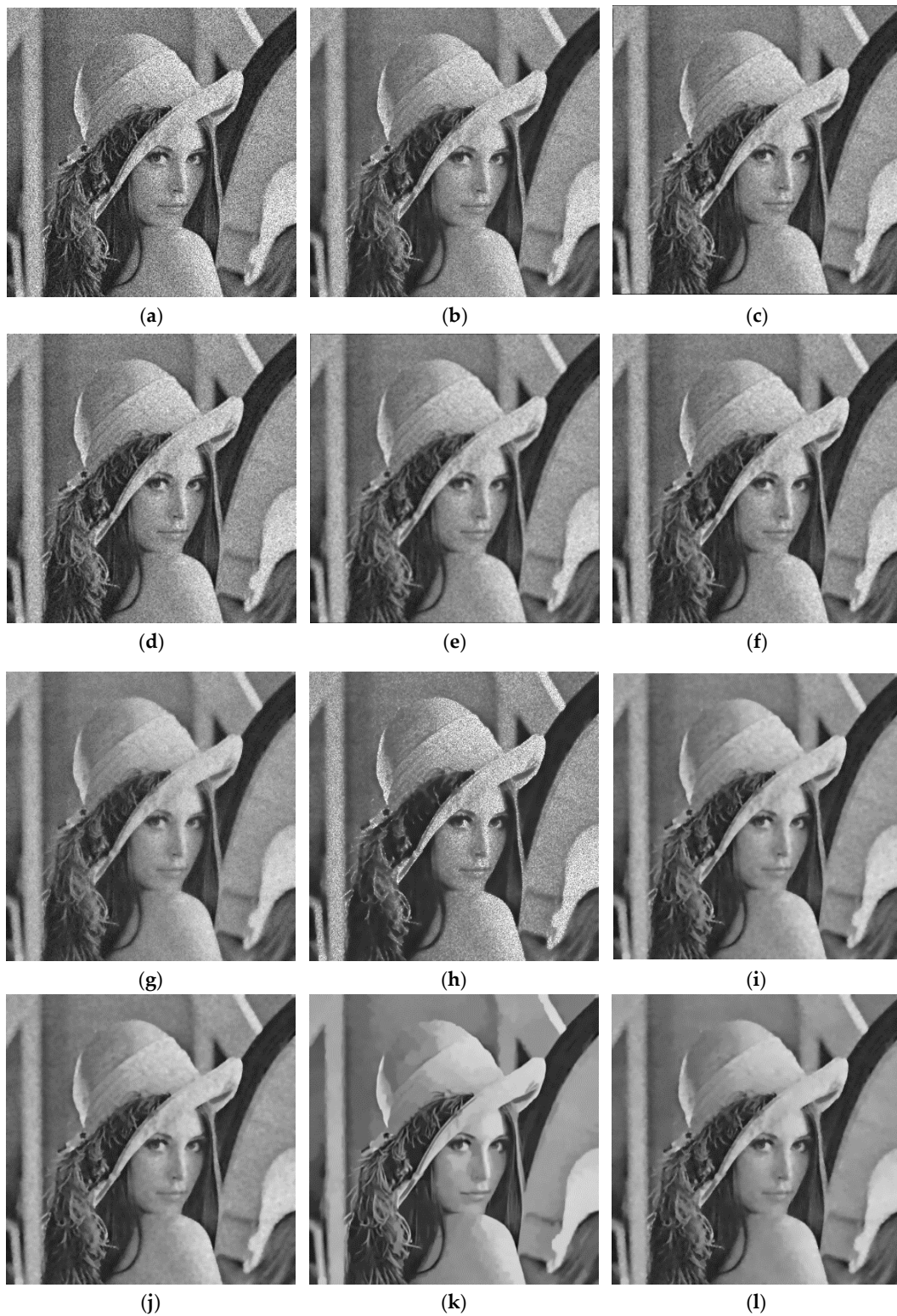
Figure 6. Despeckled results of Lena image at speckle noise \sigma = 0.04 : (a) Noisy image; (b) GIF; (c) Lee filter; (d) Frost filter; (e) Gaussian filter; (f) Bitonic filter; (g) WLS filter; (h) ADMSS; (i) SRAD filter; (j) SRAD-Bayes method; (k) SAR-BM3D; (l) Proposed algorithm.
