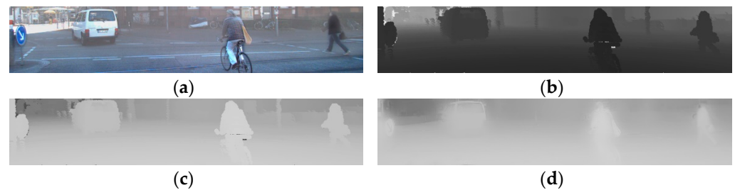
Figure 11. Refine transmission image: (a) hazy image; (b) grayscale depth image generated from point cloud projection; (c) raw transmission image from grayscale depth image; (d) refined transmission image.
