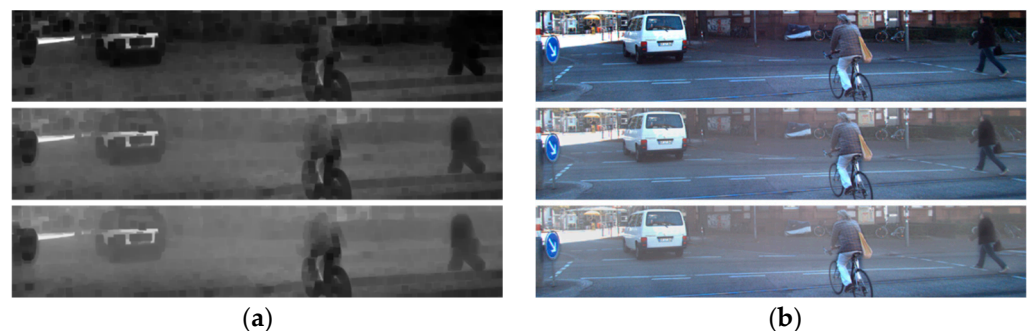
Figure 8. Generated dark channel depending on different intensity of haze: (a) dark channel; (b) hazy image.
