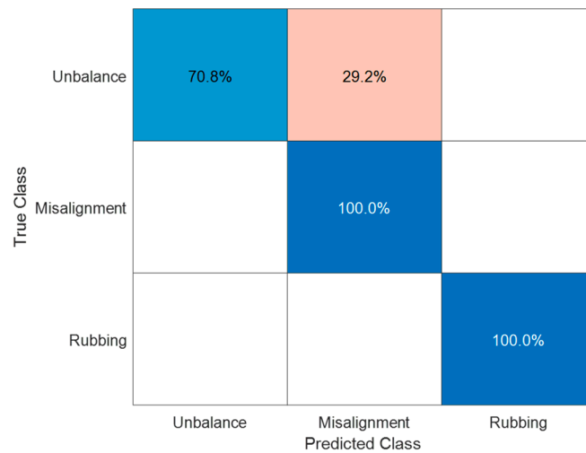
Figure 8. Test confusion matrix showing the performance of the pretrained deep learning model on unseen simulation test data (90.27% accuracy on test data).
