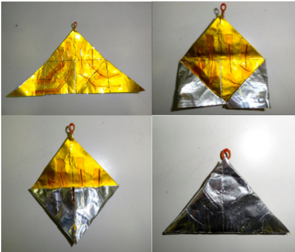
Figure 10. Folding configuration of self-deployed solar sail [123] Reproduced with permission from MDPI under STM Permissions Guidelines.
