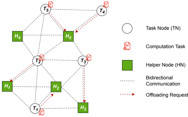
Fig. 1. An illustrative model of FCN with two types of FNs including TNs and HNs.
