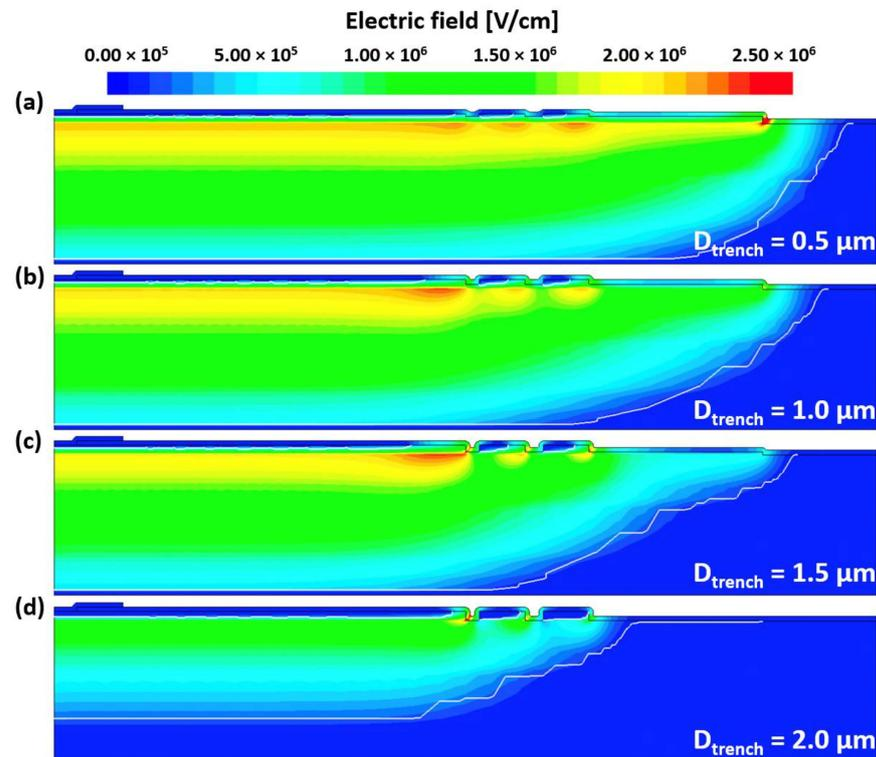
**Figure 14.** Electric field distributions of TRA-JTE with  $D_{\text{trench}}$  values of (a) 0.5  $\mu\text{m}$ , (b) 1.0  $\mu\text{m}$ , (c) 1.5  $\mu\text{m}$ , and (d) 2.0  $\mu\text{m}$  at  $N_{\text{JTE}}$  value of  $7 \times 10^{16} \text{ cm}^{-3}$ .
