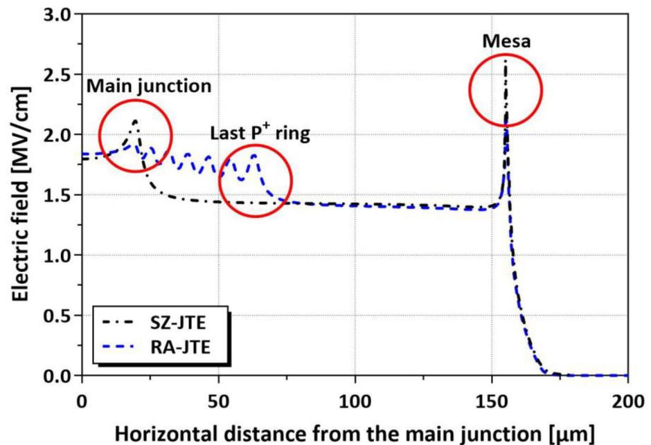
Figure 4. Electric field distributions of SZ-JTE and RA-JTE at reverse bias of 3.0 kV for  $N_{JTE}$  value of  $4 \times 10^{16} \text{ cm}^{-3}$ .
