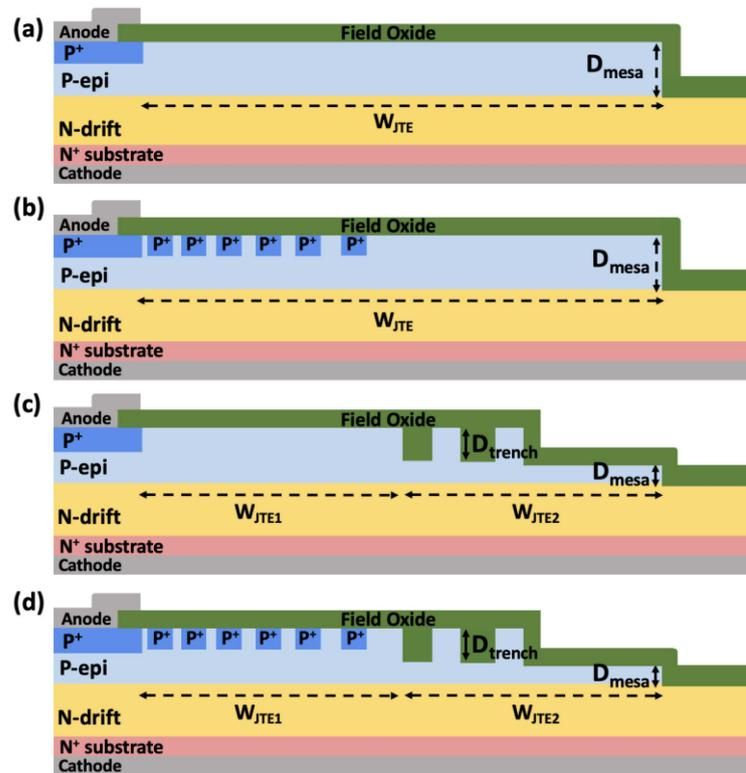
Figure 1. Cross-sectional views of (a) SZ-JTE, (b) RA-JTE, (c) T-JTE, and (d) TRA-JTE.
