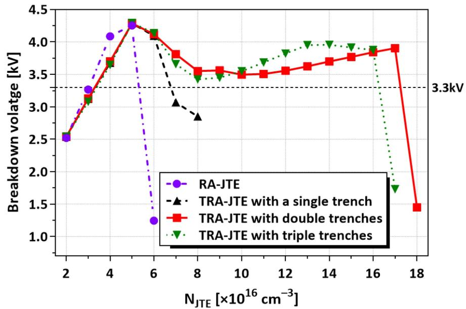
Figure 12. BVs according to  $N_{JTE}$  and  $N_{trench}$  for RA-JTE and TRA-JTE with identical  $D_{trench}$  of 1.5  $\mu\text{m}$ .
