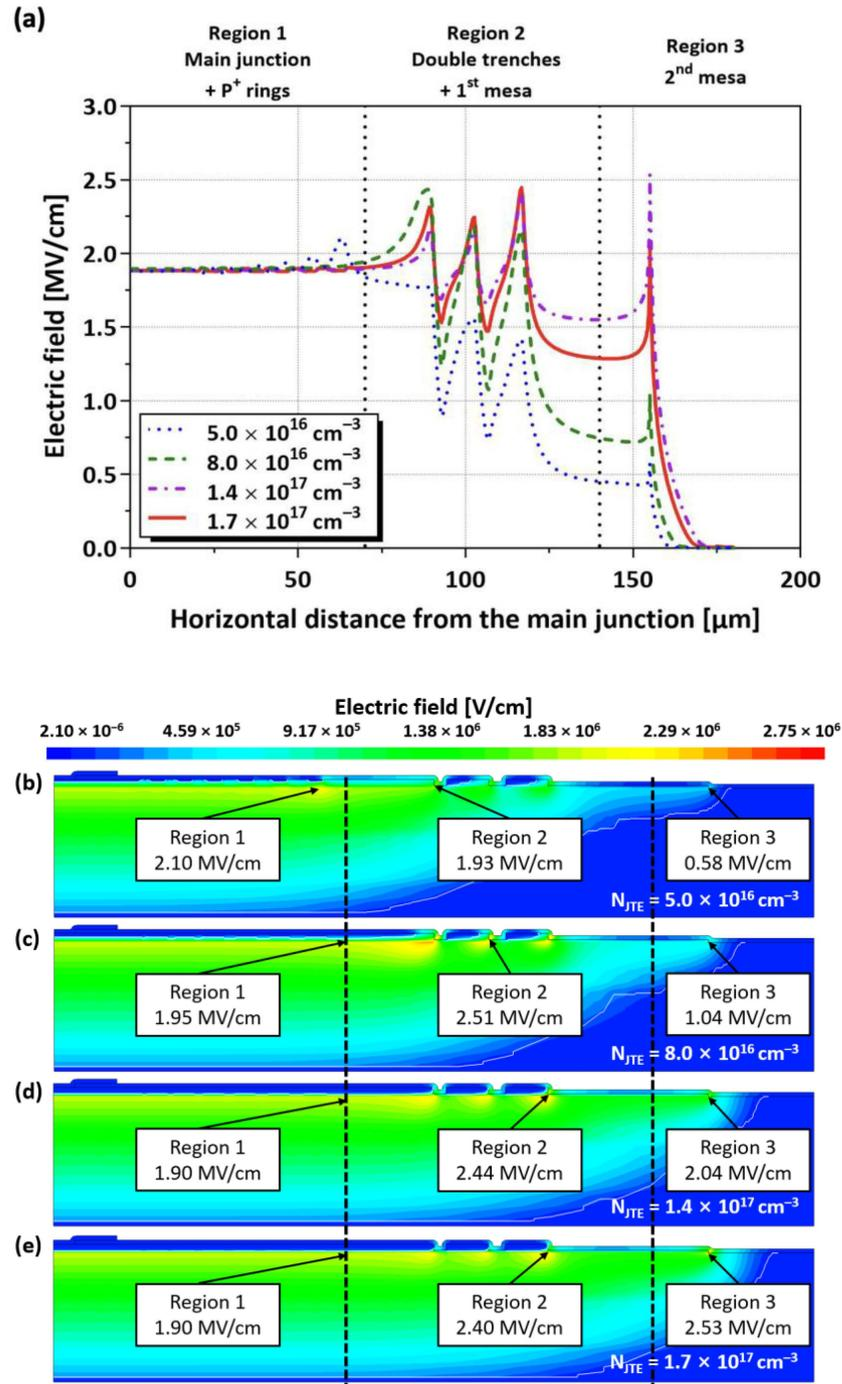
**Figure 8.** (a) Electric field distributions for TRA-JTE at reverse bias of 3.3 kV with various  $N_{JTE}$  and peak electric field of TRA-JTE per divided region for  $N_{JTE}$  values of (b)  $5 \times 10^{16} \text{ cm}^{-3}$ , (c)  $8 \times 10^{16} \text{ cm}^{-3}$ , (d)  $1.4 \times 10^{17} \text{ cm}^{-3}$ , and (e)  $1.7 \times 10^{17} \text{ cm}^{-3}$ .
