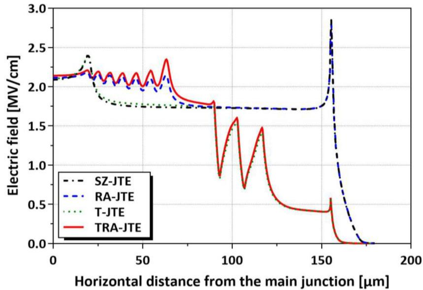
Figure 9. Electric field distributions of SZ-JTE, RA-JTE, T-JTE, and TRA-JTE at breakdown for  $N_{JTE}$  value of  $5 \times 10^{16} \text{ cm}^{-3}$ .
