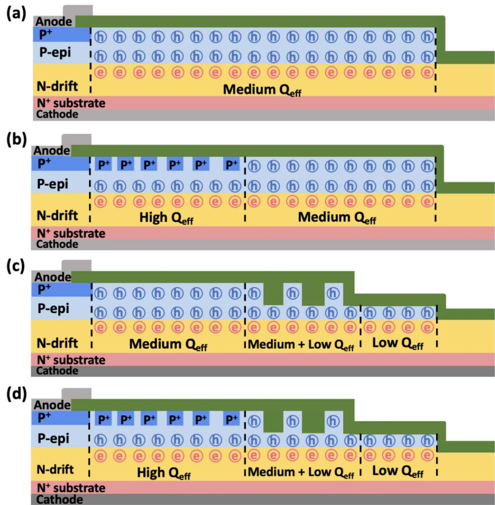
Figure 7. Cross-sectional views of  $Q_{eff}$  including electrons and holes per unit area for (a) SZ-JTE, (b) RA-JTE, (c) T-JTE, and (d) TRA-JTE.
