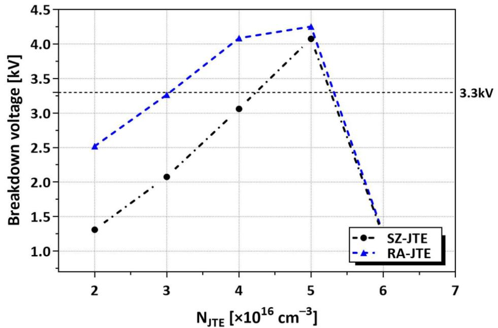
Figure 3. BVs according to  $N_{JTE}$  for SZ-JTE and RA-JTE.  $N_{JTE}$  values are increased by  $1 \times 10^{16} \text{ cm}^{-3}$  from  $2 \times 10^{16} \text{ cm}^{-3}$  to  $6 \times 10^{16} \text{ cm}^{-3}$ .
