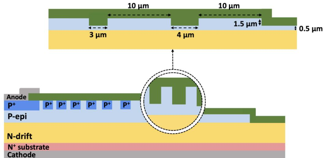
Figure 2. Widths and spaces between double trenches of TRA-JTE.
