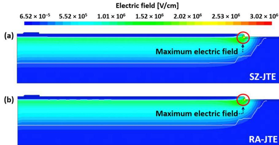
Figure 5. Electric field distributions of (a) SZ-JTE and (b) RA-JTE at reverse bias of 1.2 kV of  $N_{JTE}$  value of  $6 \times 10^{16} \text{ cm}^{-3}$ .
