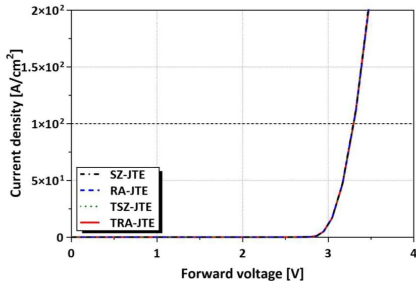
Figure 10. J–V characteristics of the SZ-JTE, RA-JTE, T-JTE, and TRA-JTE for the  $N_{JTE}$  value of  $5 \times 10^{16} \text{ cm}^{-3}$ .
