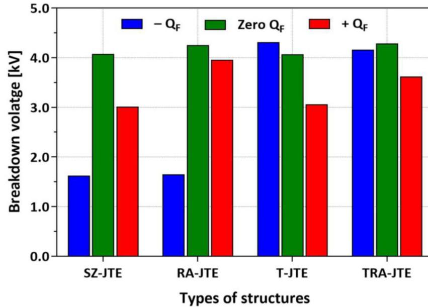
**Figure 11.** BVs according to  $Q_F$  of  $\pm 2 \times 10^{12} \text{ cm}^{-2}$  for SZ-JTE, RA-JTE, T-JTE, and TRA-JTE at  $N_{JTE}$  value of  $5 \times 10^{16} \text{ cm}^{-3}$ .
