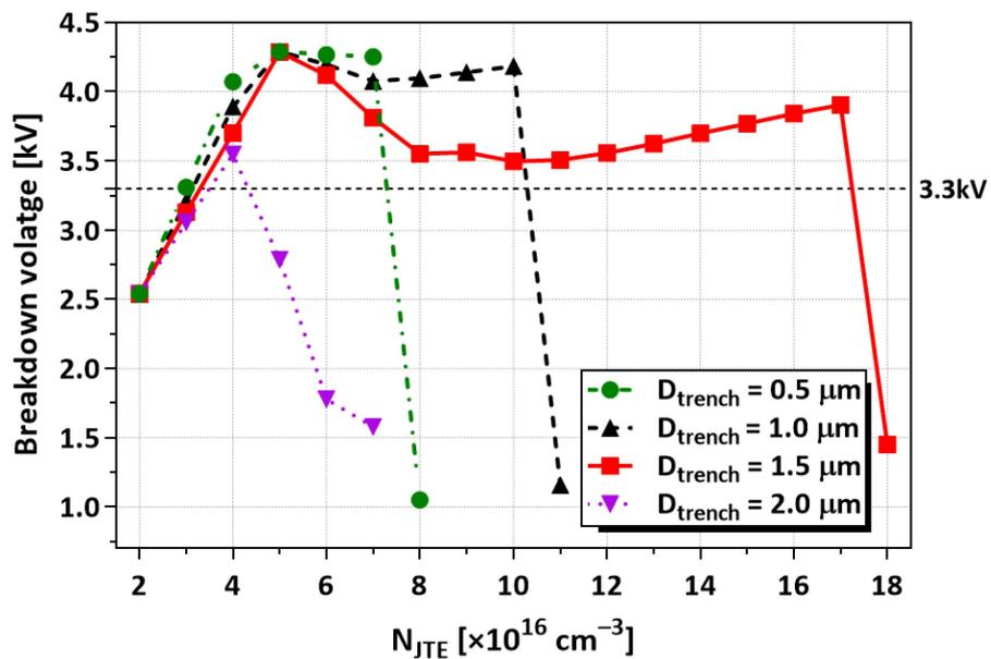
Figure 13. BVs according to  $N_{JTE}$  and  $D_{trench}$  for TRA-JTE with double trenches.
