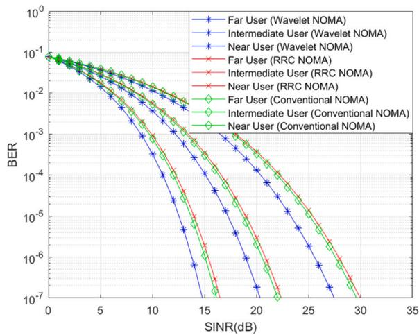
Fig. 5. BER vs. SINR in CF-mMIMO system using MMSE method for CE with pilot contamination.
