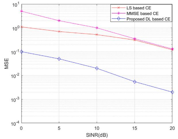
Fig. 3. MSE vs. SINR for CF-mMIMO system with wavelet NOMA scheme using LS, MMSE and DL based CE.
