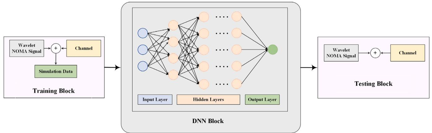
Fig. 2. DNN structure for wavelet NOMA scheme.
