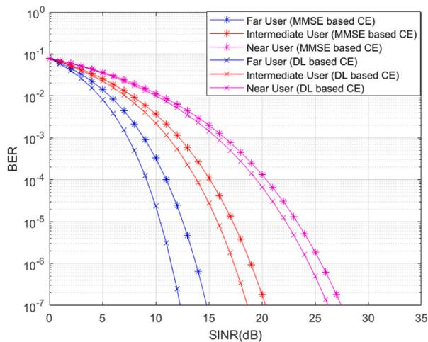
Fig. 6. BER vs. SINR for wavelet NOMA based CF-mMIMO system with pilot contamination.
