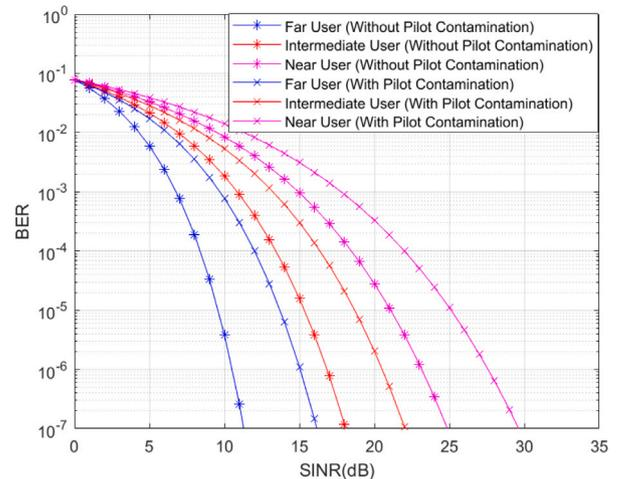
Fig. 4. BER vs. SINR in CF-mMIMO system with conventional NOMA using MMSE method for CE.
