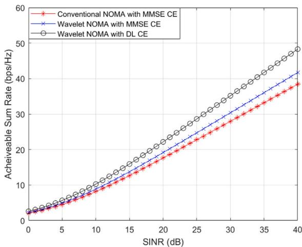
Fig. 9. Achievable sum-rate vs. SINR of CF-mMIMO system with pilot contamination.
