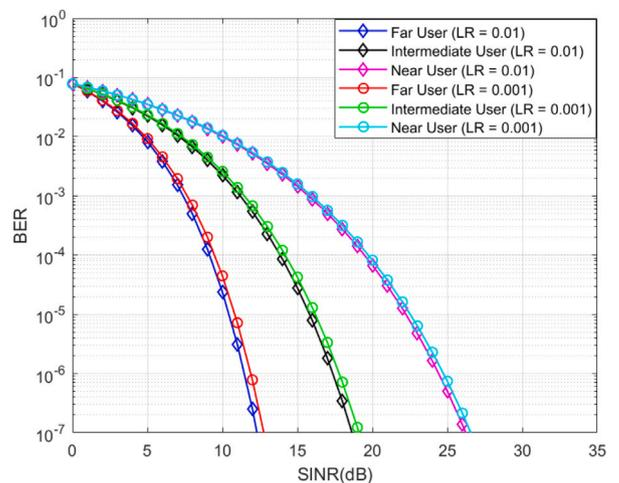
**Fig. 14.** BER vs. SINR of the proposed system with different LR.
