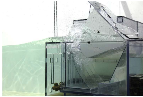
Figure 12. A view of the flood barrier erection during the wave action when h = 0.45 m. The barrier was almost fully erected. The wave hit the front face of the barrier, causing significant pressure to be applied on the pressure transducers located there.
