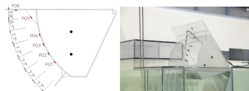
Figure 6. A diagram illustrating the location of the six pressure transducers and a picture showing how they are installed on the model.
