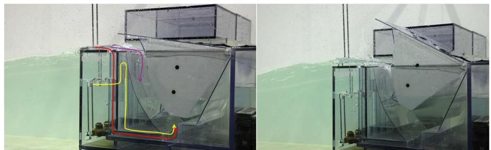
Figure 10. A view of the flood barrier erection during the wave action when h = 0.4 m. The left and right panel shows the appearance after about 40 s and 50 s after wave generation, respectively. The water levels in the rear chamber of the two panels show a clear difference. In the left panel, the yellow and red arrows indicate the flow direction through the internal and external inlets, respectively. The waterway connected to the external inlet is positioned near the glass wall, whereas the waterway connected to the internal inlet is located toward the center of the flume. The purple arrow indicates the water flow falling directly into the rear chamber along the front surface of the flood barrier.
