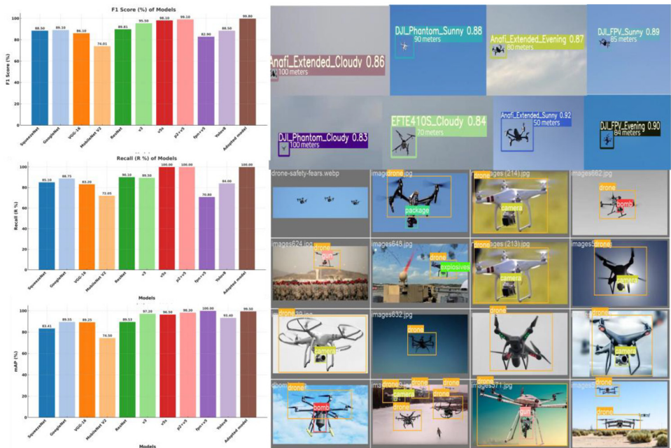
Fig. 7. (Left:) Detection performance of various object detection models on VisioDECT. (Right:) Drone Detection samples by DRONET for various UAVs at different heights and scenarios [16].
